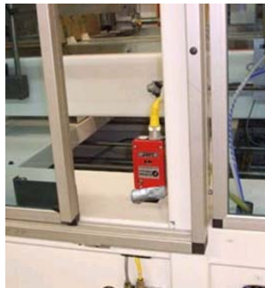
Electrical interlock taped back
