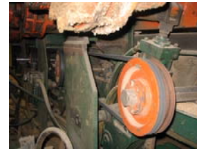
Guard not replaced after maintenance
