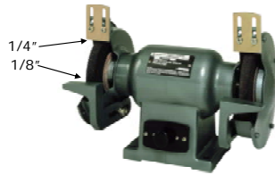
Bench Grinder w/ Adjustable Tool Rests & Tongue Guards
